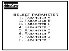
After '2' is pressed and released, the SELECT PARA-METER screen appears. Pressing the number on the screen that is associated with the desired parameter tells the RE Qualifier to load a the new parameter set and use it when monitoring fastening processes and batch counting.
