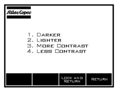
Once '9' has been pressed and the ADJUST LCD screen is in view, the brightness of the screen can be controlled by pressing keys '1' and '2'. The contrast may also be adjusted by pressing keys '3' and '4'.
