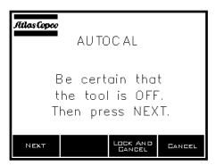
The first screen in the AutoCal<sup>TM</sup> process will say, "AUTOCAL .. Be certain that the tool is OFF. Then press NEXT.". At this point be sure the pressure transducer is connected to both the tool and to the RE Qualifier and push the soft-key labeled NEXT.
