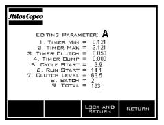
Choosing '1. Edit Parameter' from the MORE OPTIONS menu allows access to timers, pressure levels, totals, and batch settings for any given parameter. In order to edit a parameter, press the 'MORE' soft-key while at the main screen.
