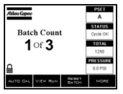
Along the right hand side of the screen, four boxes appear vertically and are labeled PSET, STATUS, TOTAL, and PRESSURE.
