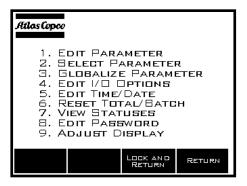
A list of nine additional functions will appear similar to the picture on the left. In order to access any of the functions on the list, press the number on the keypad that is associated with the desired function from the list.
