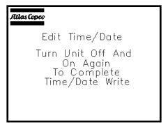
After '5' is pressed and released, the EDIT TIME/DATE screen appears. Pressing the number on the screen that is associated with the desired time/date value alters that value.
