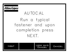
During this process, run the fastener completely allowing the tool's clutch mechanism to turn off the tool. If you make a mistake during this part of the process, run another fastener. The RE Qualifier will use the very last fastening process it sees as the basis for the calibration.
