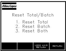
After '6' is pressed and released, the RESET TOTAL/BATCH screen appears. Pressing the number on the screen that is associated with the total, batch, or both resets that value to zero.
