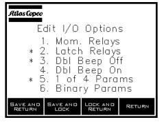
After '4' is pressed and released, the EDIT I/O OPTIONS screen appears. Six setting are listed on this screen. Pressing the number next to a desired setting will select that setting. Each setting that is active will have an asterisk (\*) in front of the number.
