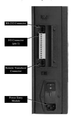
connector. Pin 1 on the connector is the top-most pin as pictured in the figure to the left. The pinout is as follows:
