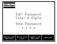
After '8' is pressed and released, the EDIT PASS-WORD screen appears. The user may type a new four digit password. As each number is entered, an asterisk (\*) will appear to represent that number. If a mistake is made, the CLR button can be used to remove one number in the password at a time (an asterisk will be removed as well).
